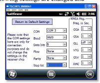
**NOTE**: The COM settings are grayed out and cannot be changed until you disconnect from your unit's GPS receiver.
