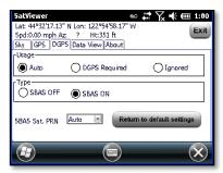
The GPS receiver used with SatViewer can provide DGPS through the Satellite Based Augmentation System (SBAS), which uses multiple ground stations and then broadcasts corrections to the end users via SBAS satellites.
