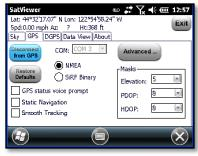
GPS receiver. Your GPS receiver port is set to COM3 and a baud rate of 9600. The default SatViewer settings shouldn't need to be changed to connect.
