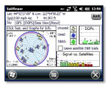
represents the horizon and the red circle represents the elevation mask. The light gray circles radiating out from the center are the zenith angles in ten-degree increments. The lines bisecting the light gray circles divide the circle into thirty-degree azimuths.
